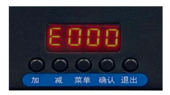
1 is to send drum data (do not forward dmx512 data) 0 is not sending drum data
