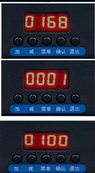
Enter the settings interface through addition and subtraction
